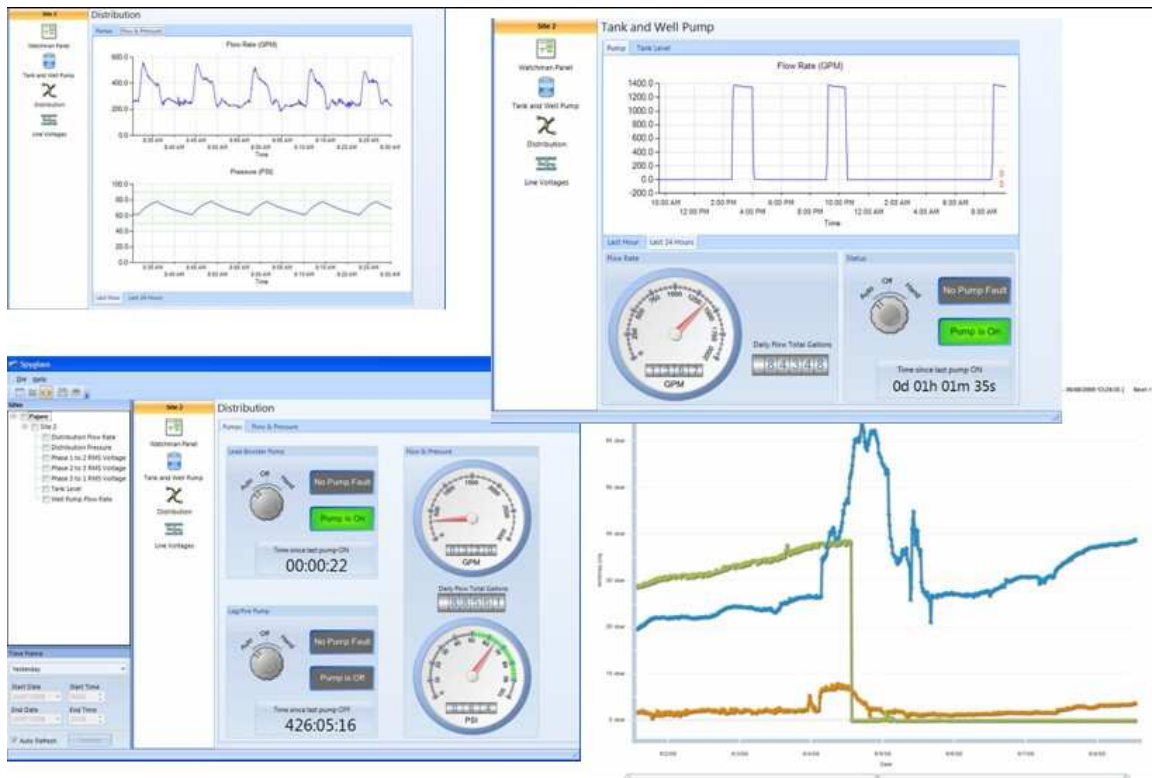
Figure 2, Control Panels and Data Trend Charts from the Saturn System of Iris Connection, Inc.
